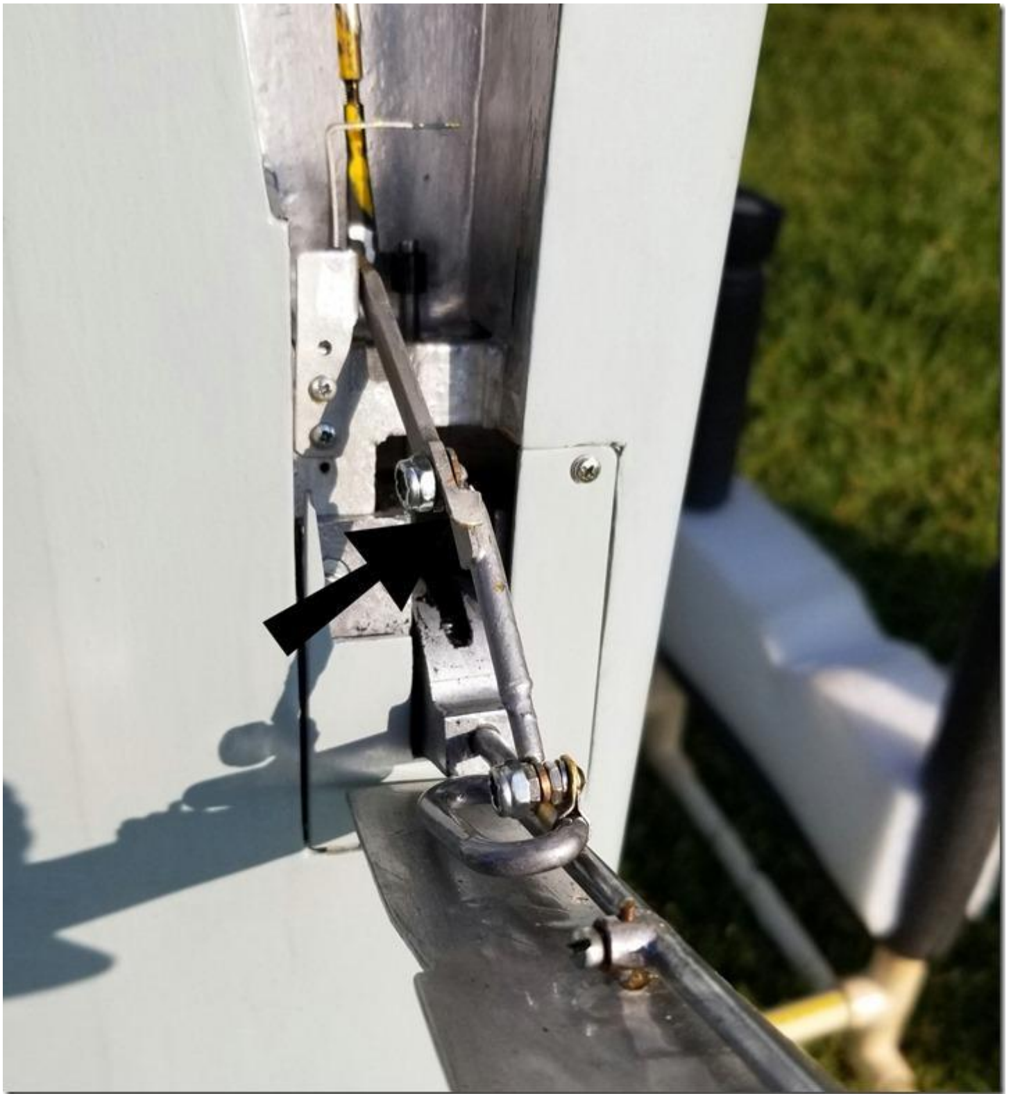
Checkout the drive linkage that operates each wheel strut: Note the overdrive stop on the folding link...
